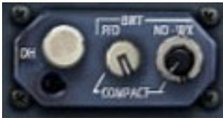
The EFIS dimming controls are only a small subpanel on the main instrument panel, and can be found to the left of the PFD. The only functional knob is the decision height knob (DH). Use it to set the decision height. Upon clicking the Decision Height will be shown in the lower right corner of the PFD.
