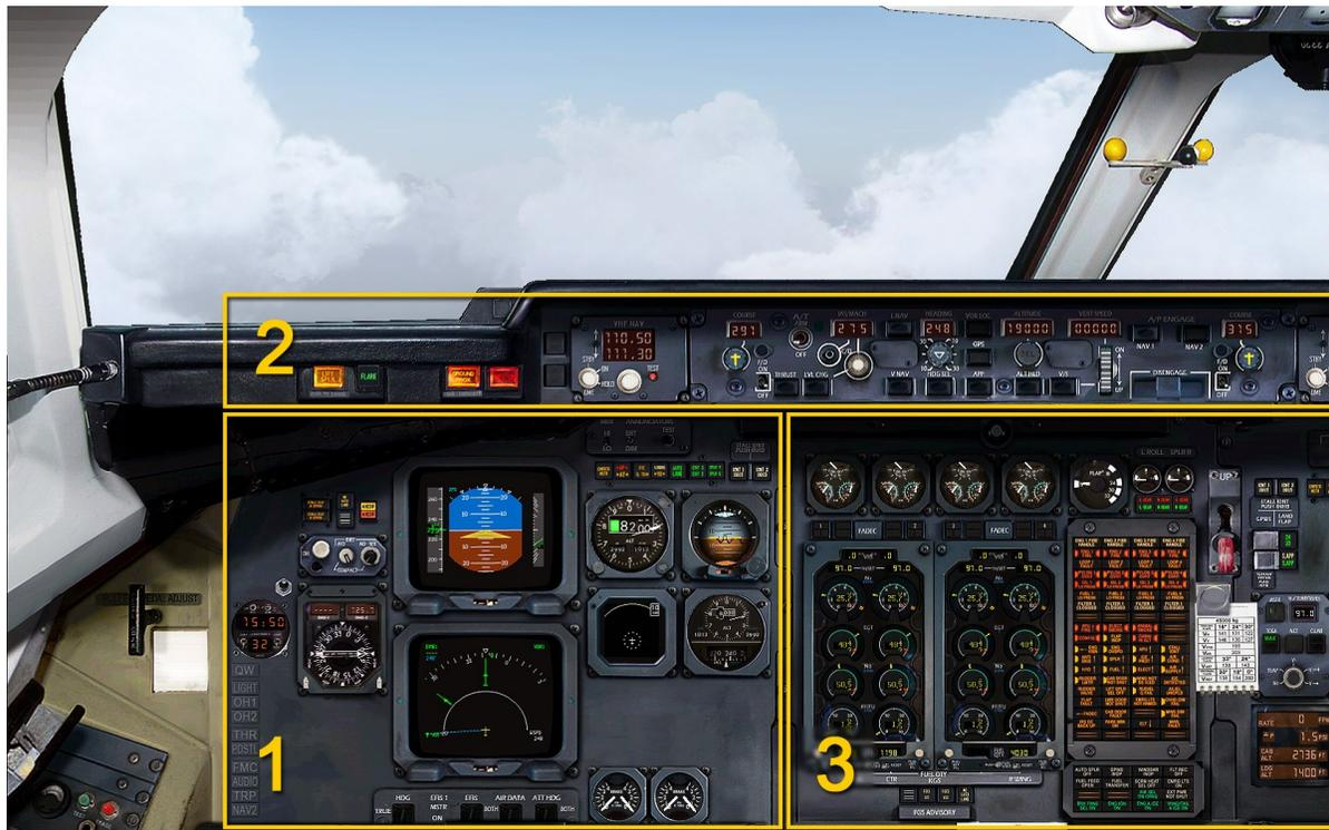
The Figure above shows this separation in functionality. You will have noticed that in this figure only three areas have been signified, and not four. This is because part of the main instrument panel is not displayed: the missing part contains the first/officer's flight instruments. Would this part be displayed, it would have been "part four". As such, we can summarize the various panels as having these functionalities:
