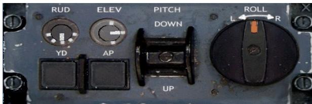
Figure XX: Autopilot Control Panel
