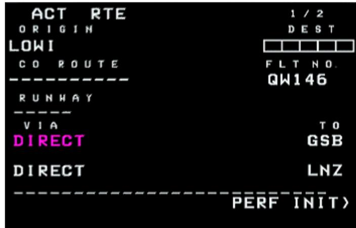
If a route is too long to be held on just page 1, additional pages are created to hold the rest of the route segments. The format is the same as on page 1 VIA/TO, as it's in principle just a continuation of the data displayed on page 1. Note the stripes in the VIA and TO columns below the last segment. These enable you to add new segments at any time manually by typing them into the scratchpad and pressing the associated line select keys.
