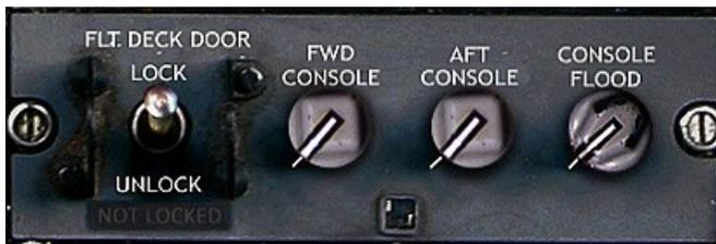
The Pedestal Lighting Controls can be found at the very aft portion of the pedestal
