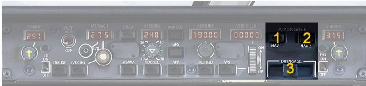
Figure 44: Autopilot engagement/disengagement controls
