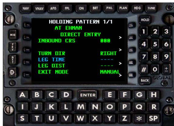
The hold feature is activated by selecting a waypoint on the Active FPL page, when the waypoint is highlighted (via the left LSK's) press the HOLD button and the HOLD page will display.
