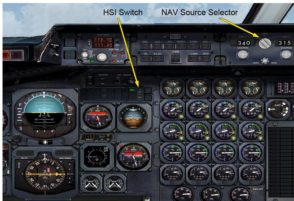
By default, the HSI switch is set to the RNAV position, which means that it is coupled up with the GNS-XLS Flight Management System. In this case the course indicator resembles the programmed track and the beam bar the lateral deviation from such. In case no flight plan is loaded, this will be indicated by a red-white flag as can be seen below.
