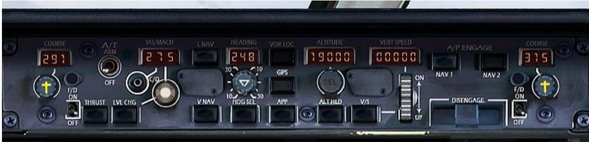
The Mode Control Panel, abbreviated to MCP, is the central location for controlling the Flight Guidance System (FGS). Here you can turn the flight directors on and off, you can select modes according to which the flight director will issue commands and you can turn the autopilot on and off.
