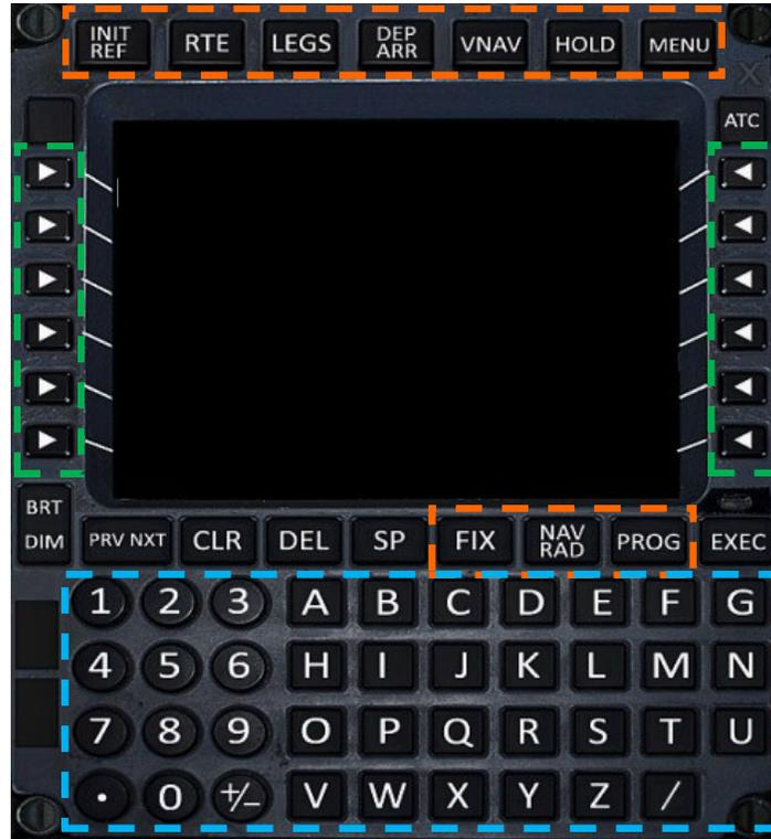
The CDU is characterized by its big display screen, which takes up the approximate top half of the CDU panel. Generally we can find three kinds of buttons on the CDU:
