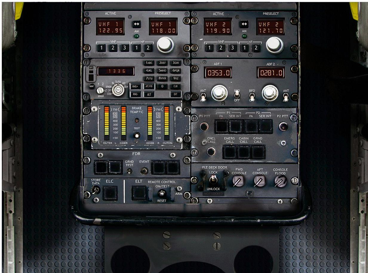
Figure 52: Radio Stack in the 2D Panel (Shift+5)
