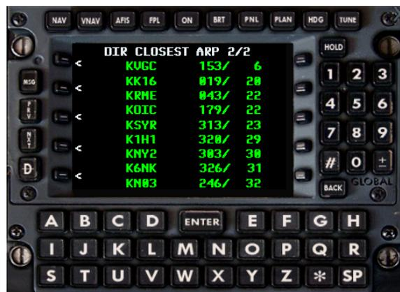
Pressing the 'D->' button until the last page is reached will display a list of the 9 nearest airports, and their bearing and distance from the aircraft's present position.
