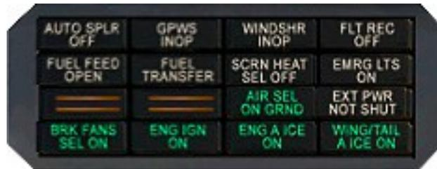
Figure 49: The Central Status Panel (CSP)
