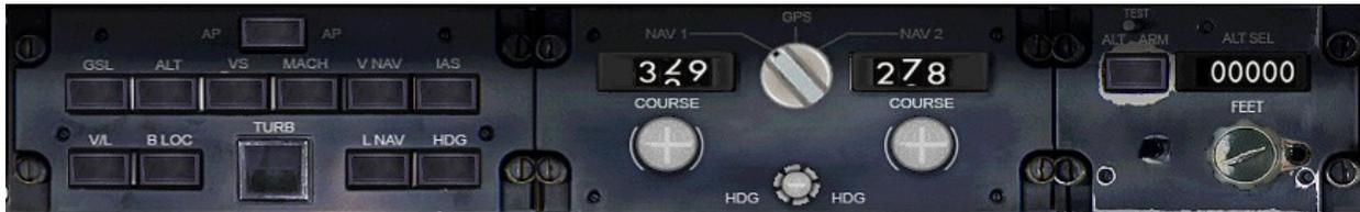
Figure XX: Autopilot engagement/disengagement controls
