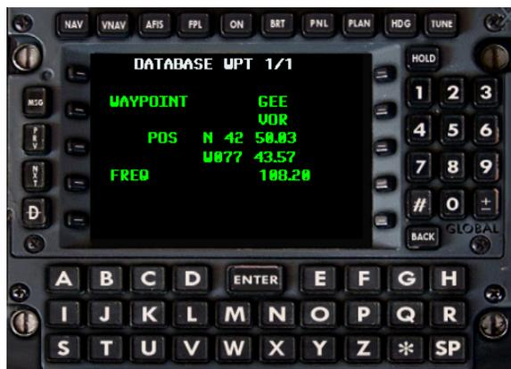
The database wpt page is displayed only when a new flight plan or direct to waypoint is entered to verify the entered identifier is indeed the navaid you wish to be inserted into the flight plan. By default the closest navaid with the same identifier to the aircraft's current position will be displayed.
