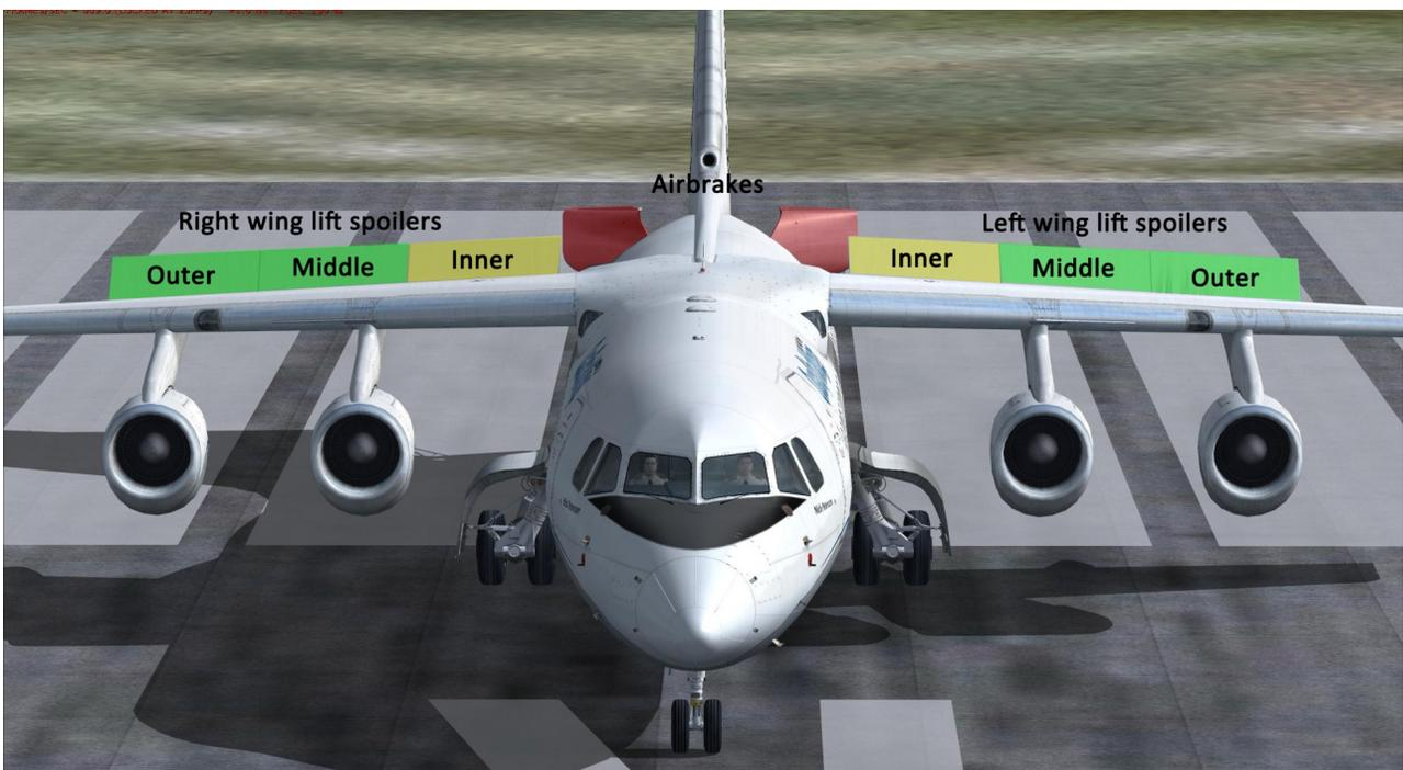
Figure 51: Lift spoilers (green/yellow) and airbrake (red) positions. The green/yellow colors on the lift spoilers signify the hydraulic system by which they are powered.
