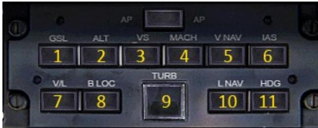
Figure 44: Autopilot engagement/disengagement controls
