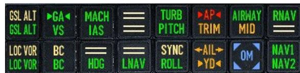
Figure XX: Flight Mode Annunciator Panel
