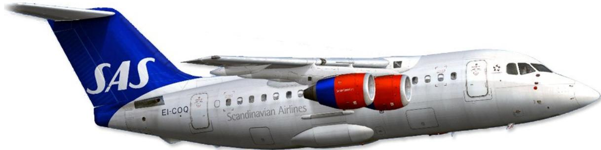
The Avro RJ70 is a modernization of the BAe146-100. Looking over the dimensions and comparing them to the BAe146-100, you might have noticed some interesting points. For example, the dimensions are exactly the same, evidence of the fact that the airframe has not been revised fundamentally in any form or part. However, you will have noticed the differences in range, weight and altitude.
