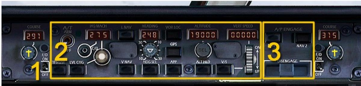
The MCP's layout probably seems cluttered and hard to understand, but within the mess there is a clear functional philosophy: all the switches that control an aspect of the FGS have been grouped together. The various button groups control the following FGS aspects (numbers in the list correspond to the numbers in the Figure above):
