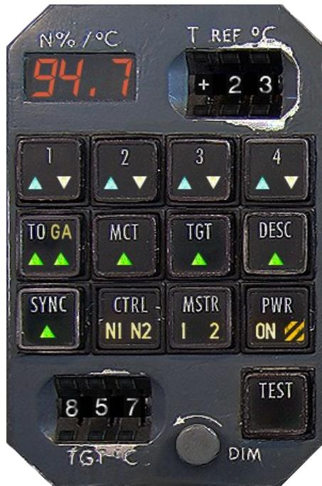
The TMS control unit consists of a LED display, showing the reference N1 percentage or the target TGT depending on the mode selected. The first row is fitted with annunciators indicating small arrows to move the thrust levers.
