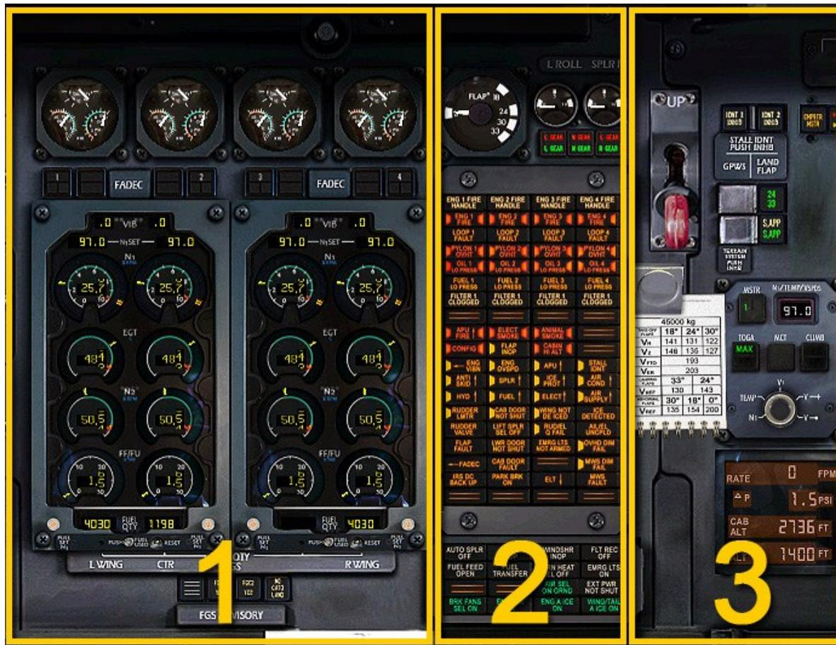
Figure 45: The engine instruments and Master Warning Panel, including some other miscellaneous stuff
