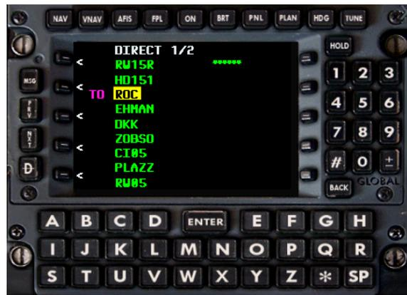
On the Direct To page, you can specify 'direct to' a Database waypoint, or 'direct to' a flight plan waypoint.
