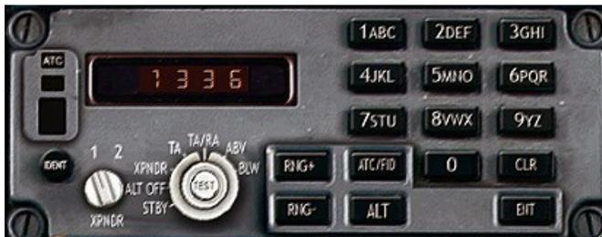
The box displayed controls both, the Traffic Collision Avoidance System (TCAS) and the aircraft's transponder. Three modes are simulated in the Ultimate 146 Collection and can be controlled using the big rotary knob below the LCD Window.
