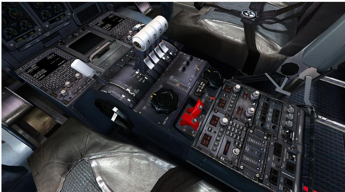
*The CDU, throttle quadrant and radio stack.*
