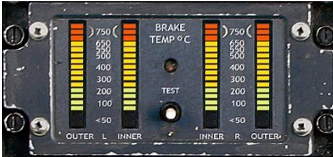
The Brake Temperature Indicator (BTI) shows the temperature of the brakes located on the main landing gear. The two indicators on the left show the brakes for the left outer and inner wheels of the main landing gear, the two indicators on the right show the brake temperature for the right outer and inner wheels of the main landing gear.
