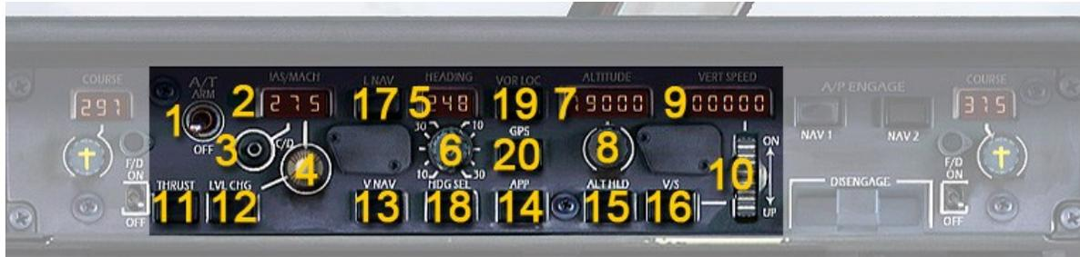
Figure 43: F/D and A/P modes on the MCP
