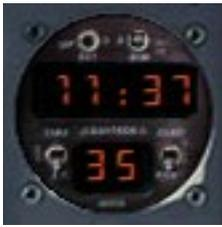
The clock is placed all the way to the left on the main instrument panel. It has two LCD screens: the upper one shows the current time; the lower one may show elapsed time. This is a basic stopwatch that can be set to run, hold or be reset.
