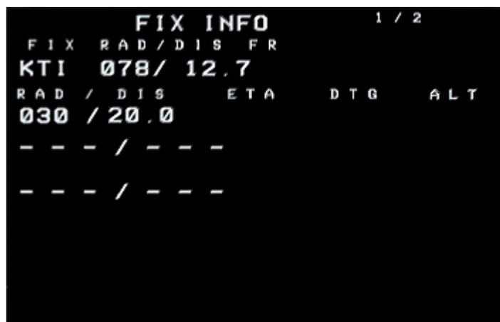
To enter a radial and distance, type both a radial in degrees, followed by a distance in nautical miles. As such you will have created a radial, and the entered distance will appear as a circle around the navigational point, which represents the entered distance from the navigational point.
