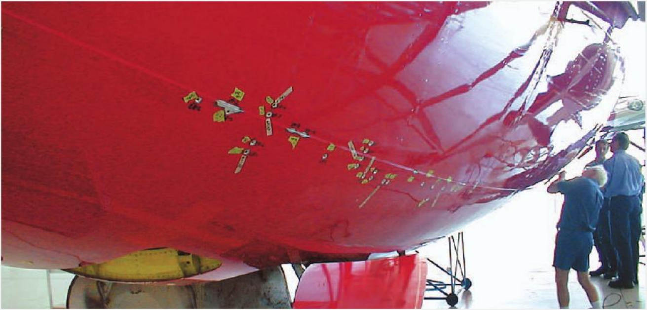
Figure 6: Damage caused by lightning moving along an airplane
